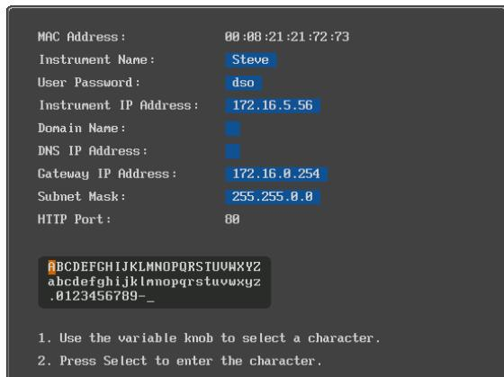
6. Use the *Up* and *Down* arrows on the side menu to navigate to each Ethernet configuration item.
